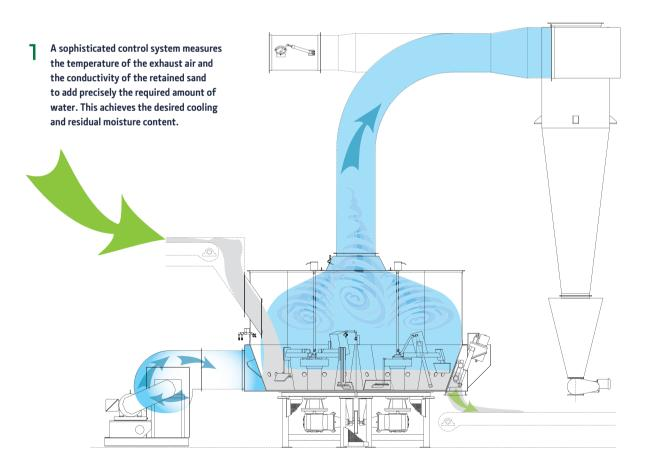
Counter-rotating mixing tool sets mechanically fluidize the retained sand so that cooling air, provided by the inlet blower, and water can be in intimate contact with the sand; thus providing for efficient and effective cooling.
