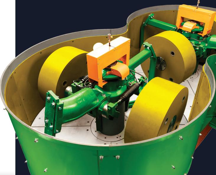
For high-volume, high-quality, cost-effective casting production, the Simpson Multi-Mull is the best solution. This technology produces larger volumes of molding sand at a lower cost of installation and operation than any other mixer in the world.
