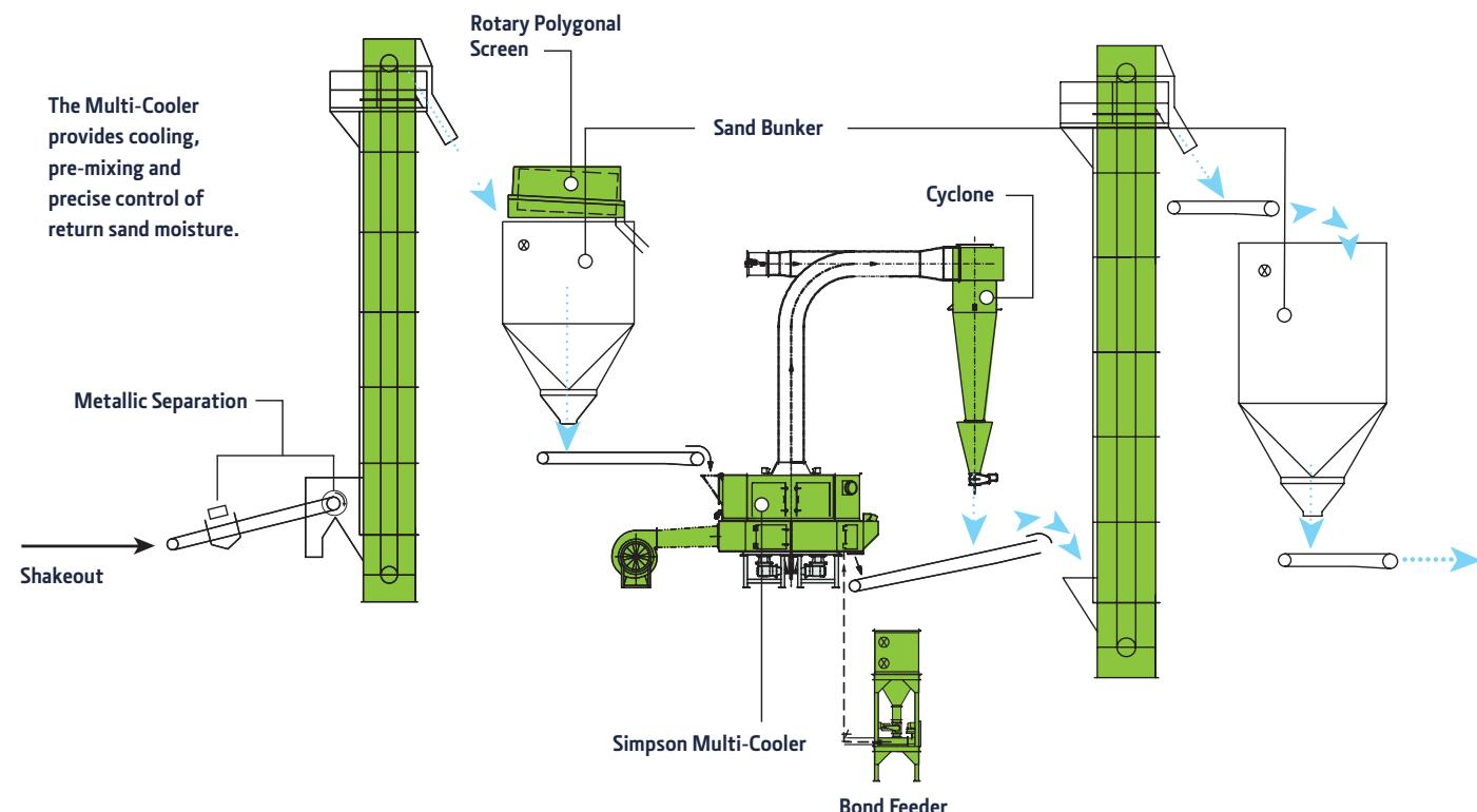
Simpson Multi-Cooler, in seven models, provides pre-mixing, cooling and moisture optimization before final mixing.
