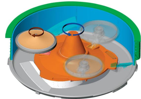
Intensive mulling in a Speedmullor is accomplished by horizontally mounted muller wheels compressing the sand against the mixer wall. Shearing and blending is provided by a series of plows mounted on the mixer crosshead. Rotating at high speed, the combination of muller wheels and plows provide full development of the bentonite and other additives.
