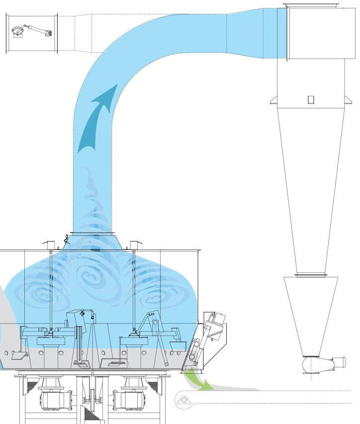
**1** A sophisticated control system measures the temperature of the exhaust air and the conductivity of the retained sand to add precisely the required amount of water. This achieves the desired cooling and residual moisture content.
