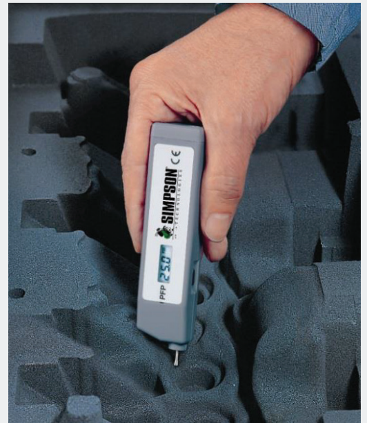
Battery-operated measuring instrument with digital readout for the determination mould strength of test specimens sand moulds.
