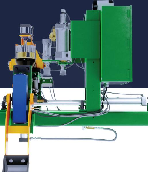
2 On discharge, the Hartley tester obtains a sample of the sand and conducts tests on the compactability, green strength (model 2552 only) and moisture. The results are compared to the desired targets and the process control logic is adjusted accordingly.
