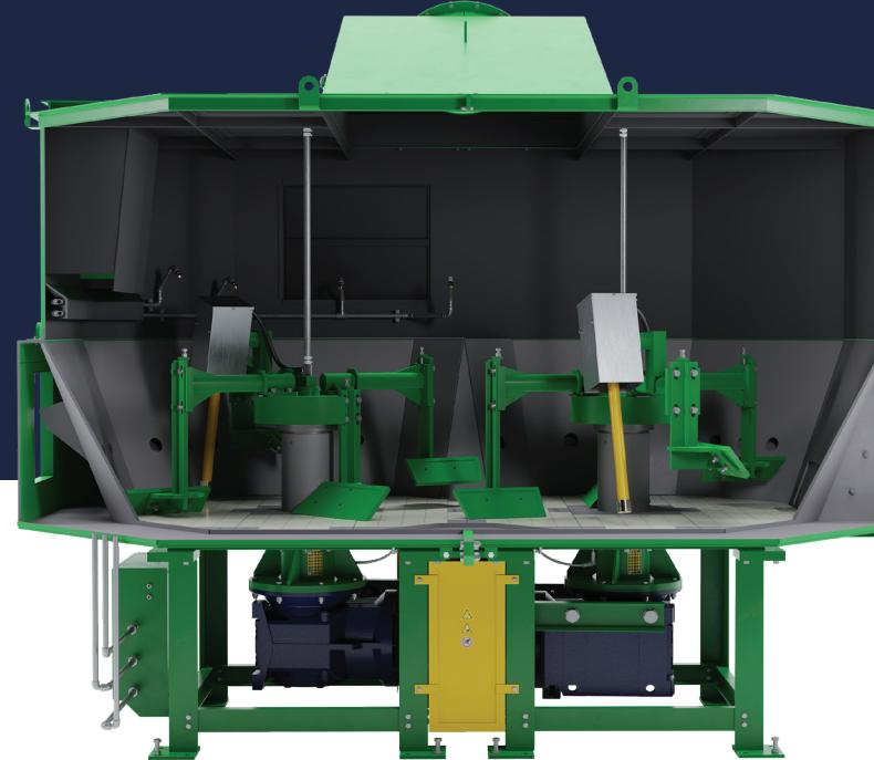
1 A sophisticated control system measures the temperature of the exhaust air and the conductivity of the retained sand to add precisely the required amount of water. This achieves the desired cooling and residual moisture content.
