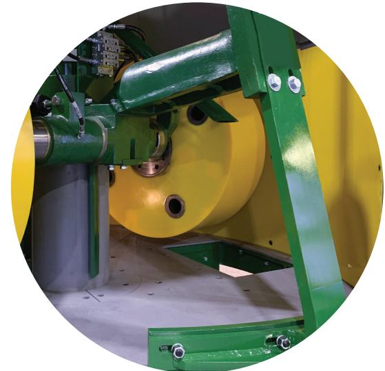
2 Interchangeable, modular plows armored with tungsten carbide provide intensive blending and minimize maintenance costs.
